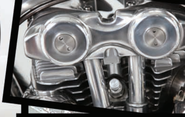
The S&S SH93 motor used in Tavax 2011V features custom rocker boxes along with a custom cam box cover and air cleaner for the S&S carb
