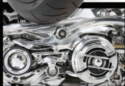
One of the few pieces on Tavax 2011V not made by Ken Tabata is the primary drive, which was sourced from Primo Rivera. However, Ken did fabricate his own belt tensioner, pulley and belt covers
